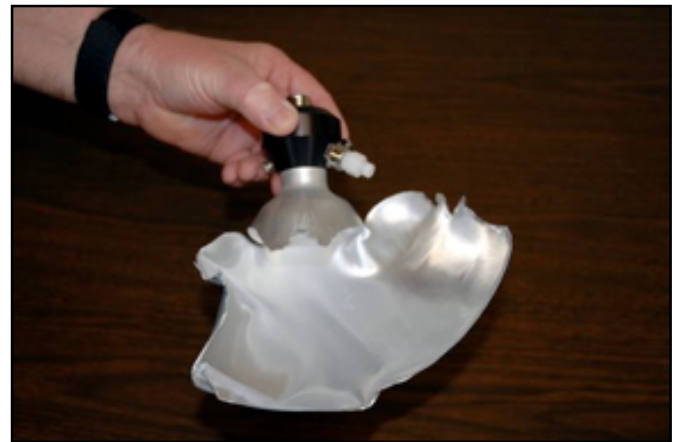
Ruptured Lawrence Factor test cylinder
