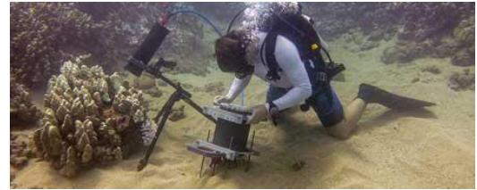
Scripps graduate student Andrew Mullen positions the Benthic Underwater Microscope to study coral competition.
